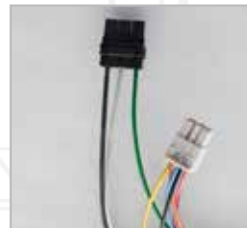
Polarized Molex Plugs Allowing for Simple Disconnect from Cabinet
